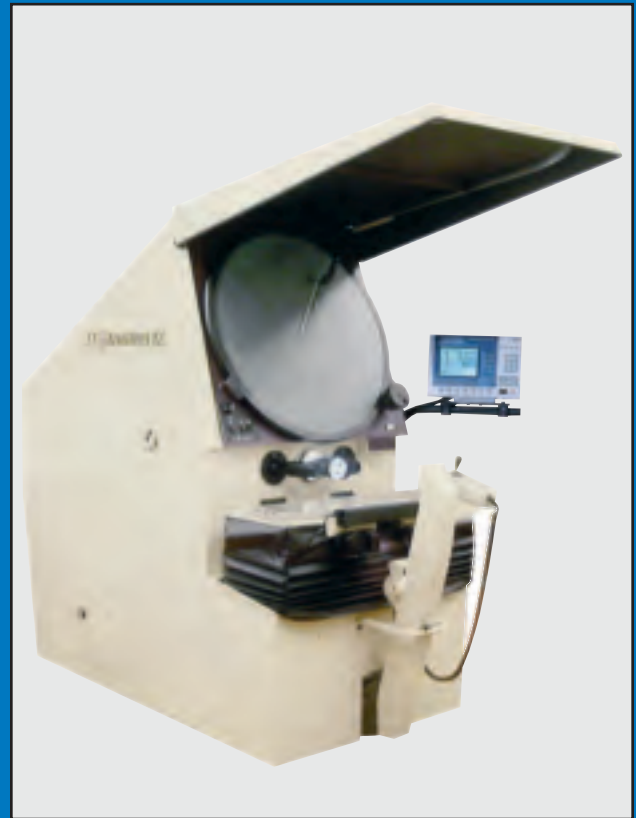
Above: Actual photo of the same 2600 Series 30" Comparator after being remanufactured at S-T Industries, ready to ship back to the customer.
